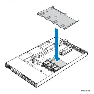
Figure 15. Installing the Processor Air Duct
